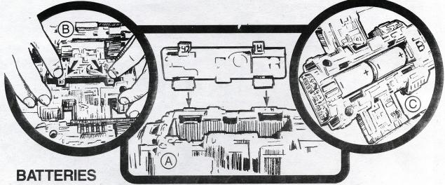
To assemble battery cover, press back hinges into position as shown. (A) Close cover to allow the two tabs to secure the door. The
